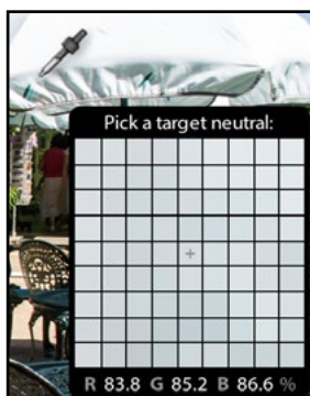
Figure 54 Select the White Balance Selector from the Basic panel and click on something that should be neutral to correct a color cast.
